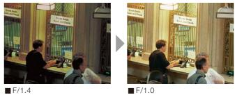
F/1.0 lens has two times light gathering power compared to F/1.4 making a 1 lux camera sensitivity into a 0.5 lux sensitivity.
